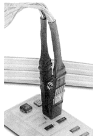
Logical Connection for Small Outline Packages (Surface Mount ICs)
