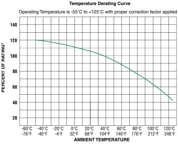
• Ambient temperature effects are in addition to the normal derating.
