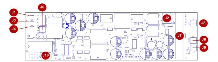
J1 = +V J2 = ATX+12V J3 = SW J4 = -V J5 = LED J6 = AMP J7 = ATX Connector J8 = Switch J9 = SwitchJ10 = Jumpers
