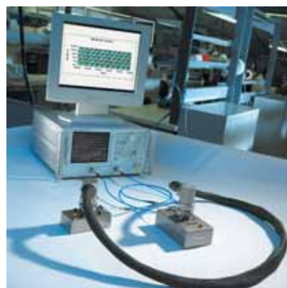
▲ MICROSTRIP INJECTION TEST BENCH TO CONTROL TRANSFER IMPEDANCE
