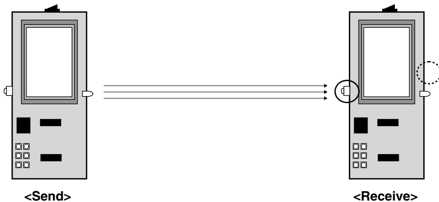
Fig. 16.1.1 Infrared Emission/Reception Evaluation Environment Using SVT17801
