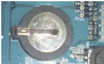
Fig. 3.4.2.2 Installing/Removing Coin Battery - 2/4
