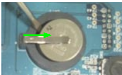
Fig. 3.4.2.4 Installing/Removing Coin Battery - 4/4
