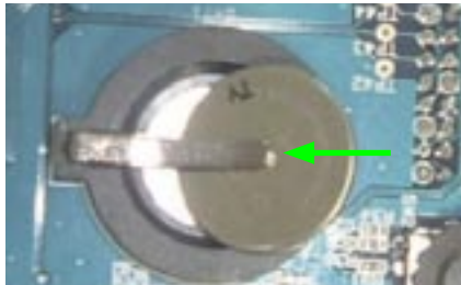
Fig. 3.4.2.1 Installing/Removing Coin Battery - 1/4
