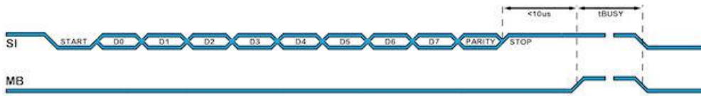
CMOS Asynchronous serial communication from host system to module. tBUSY occurs when the module receive buffer
