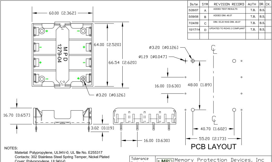
Cover: Polypropylene, UL94V-0 Heat Deflection Temperature: 90°C
