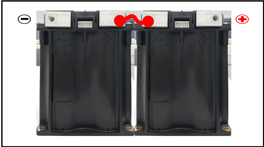
<Fig. 2> Series Connection of Modules
