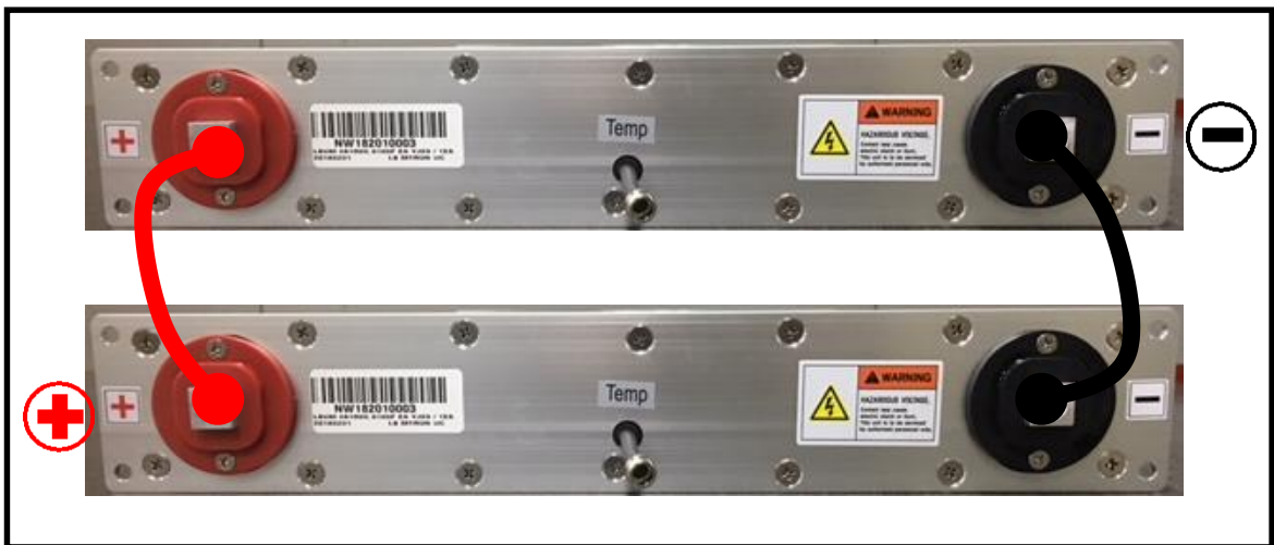
<Fig. 3> Parallel Connection of Modules.
