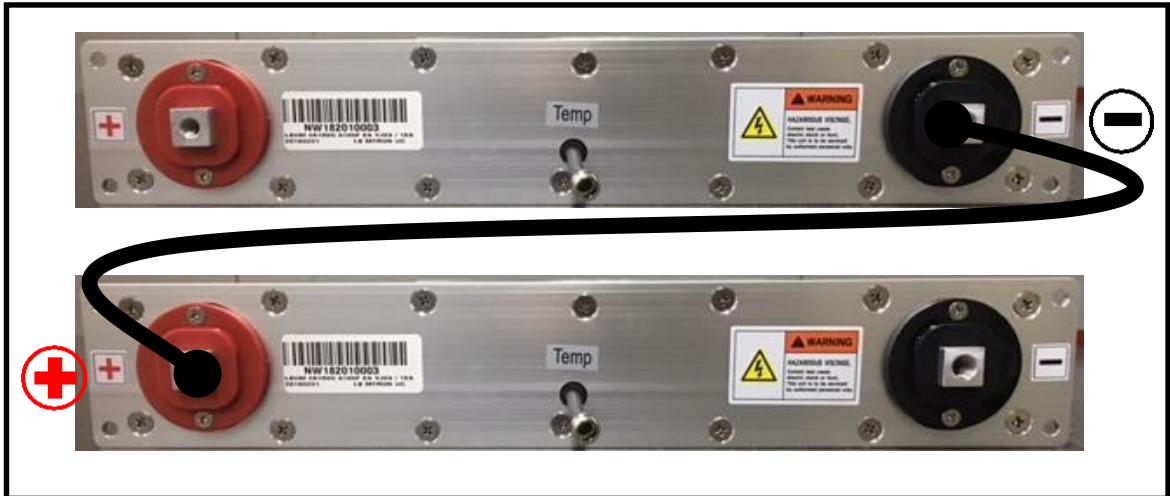
<Fig. 2> Series Connection of Modules
