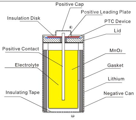
Bobbin structure, laser-sealing
