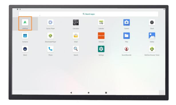
Method B: Install APK with installer app from EBOX-IMX8MM directly.
