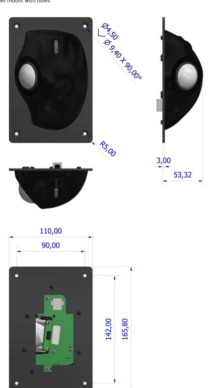
Dimensional drawing specifies factory default orientation. All dimensions are in mm unless otherwise stated. Tolerances +/- 0.25mm unless otherwise stated IGES/STEP model available on request.
