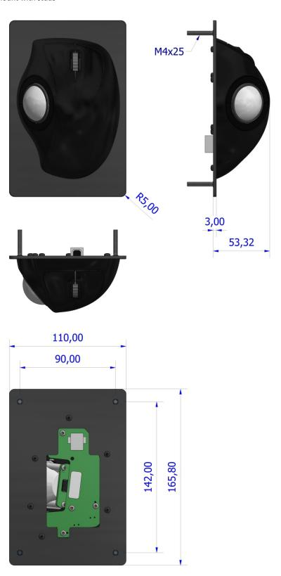
Dimensional drawing specifies factory default orientation. All dimensions are in mm unless otherwise stated. Tolerances +/- 0.25mm unless otherwise stated IGES/STEP model available on request.
