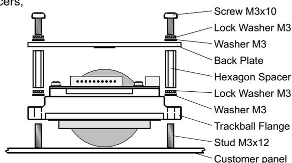
Fig. 1 : assembly procedure
