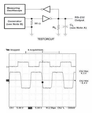
Figure 1. ZT32xxE TxIN to TxOut (no load) at 250kbps waveform
