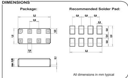
Ultra small SMT ceramic package with integrated 32.768kHz Crystal I<sup>2</sup>C Interface Address: D0h Frequency-Offset Trimming Register Programmable Alarm and Interrupt Oscillator Fail Detection Watchdog Timer Programmable Clock-Output Time keeping mode down to 1.0 V
