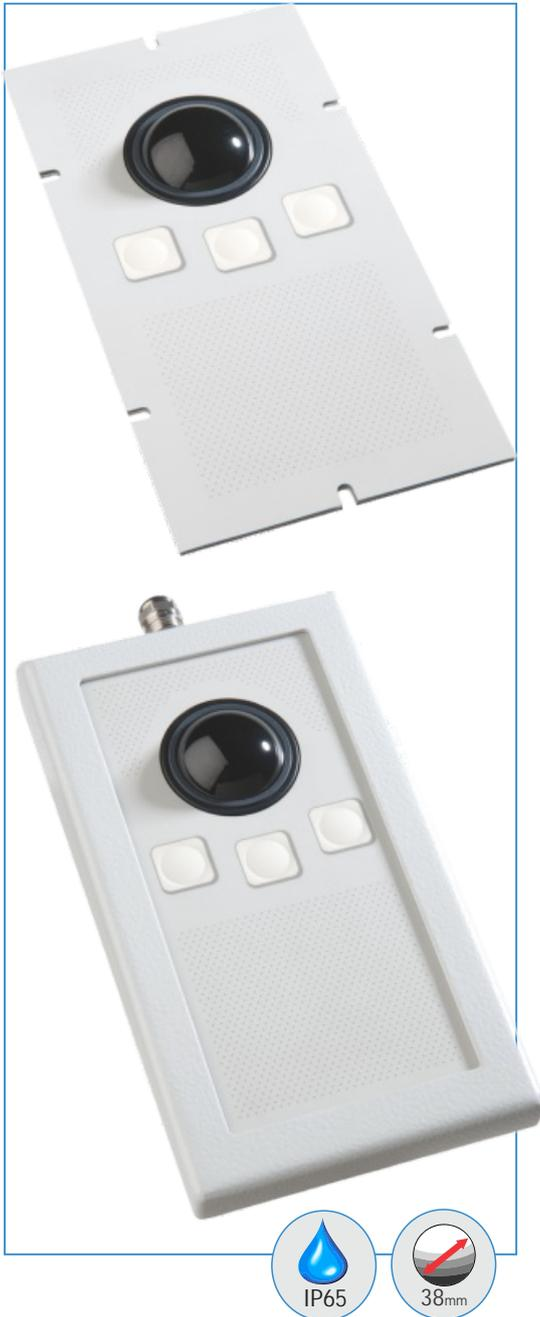
The TBM34 series is a ruggedised professional trackball. The unit has been specially designed for harsh industrial environment applications : the self-adjusting PTFE seal of the trackerball guarantees an IP65 static (ball in rest) protection grade. Carrier plates and housing are metal (aluminium and steel).
