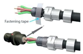
2. Strip the cable and conductors. Fold back the shield and use fastening tape to fasten it to the cable jacket. Tin-plate this wires if needed.
