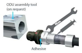
4. Screw the crimp adapter on so that it is flush, observing torque values. Secure the screw thread with adhesive. Encapsulate the interior of the crimp adapter to secure the soldered points.
