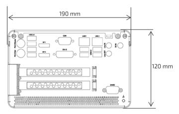
Figure 46: Dimensions Bottom Side
