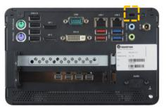
4. Remove the two top cover screws on the rear panel and retain the screws for later use.
