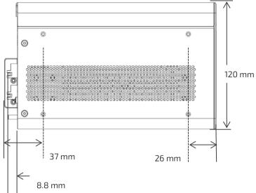
Figure 49: Dimensions with Mounting Brackets
