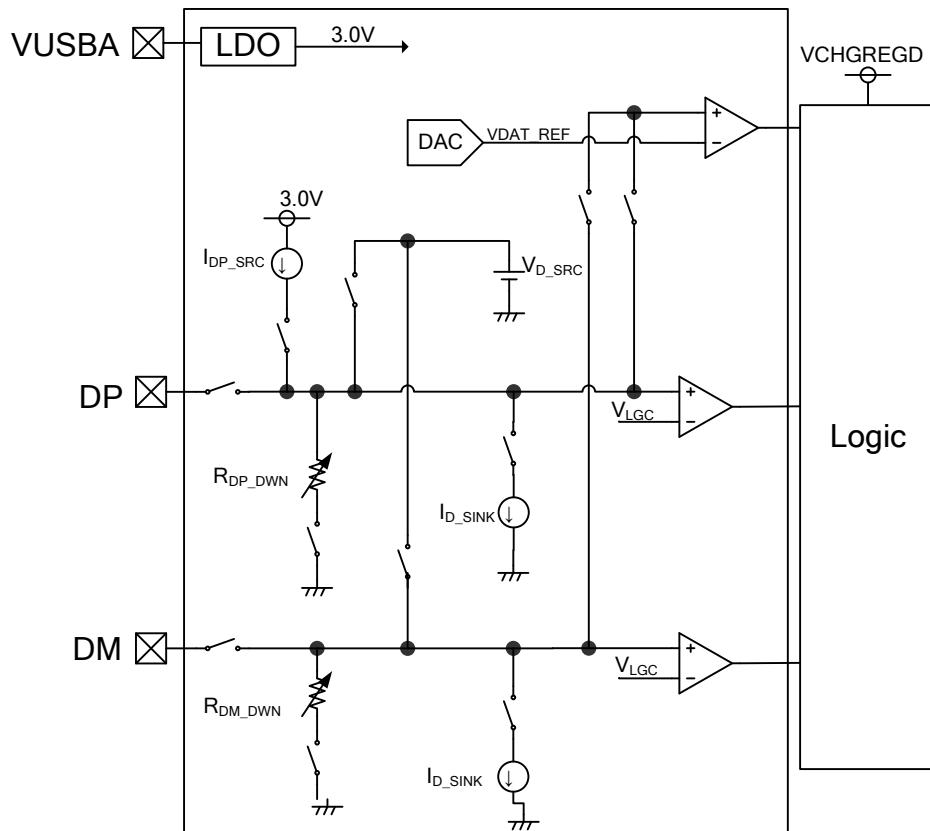
Fig 10-1 USB External Device Interface Block diagram
