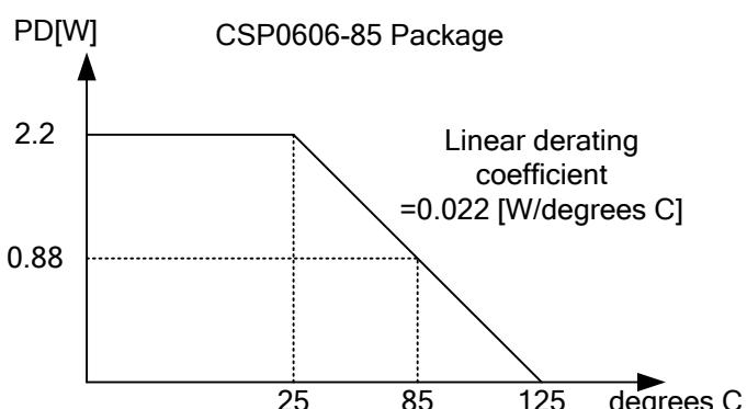
Fig 4-1 Maximum Package Allowable Dissipation
