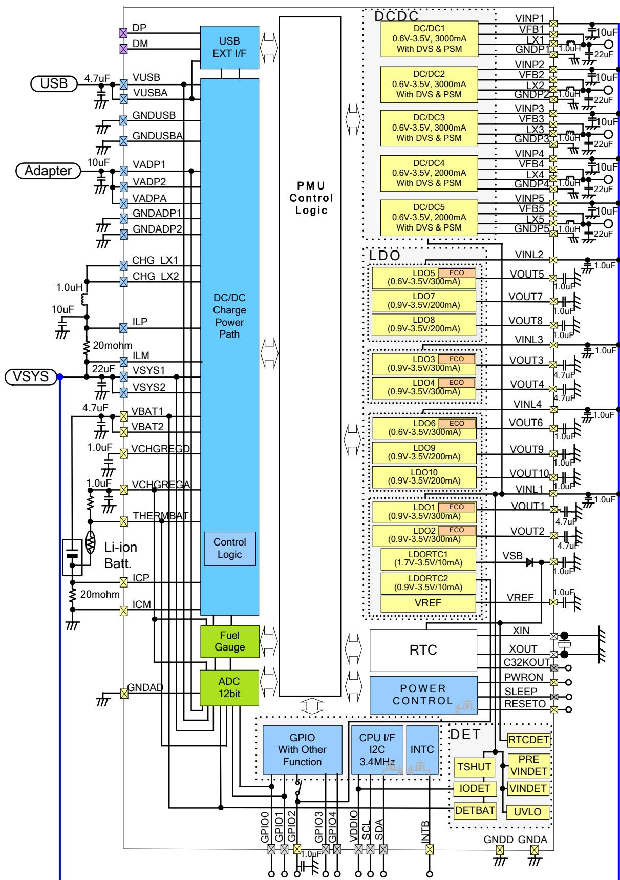
Fig 3-1 Block Diagram
