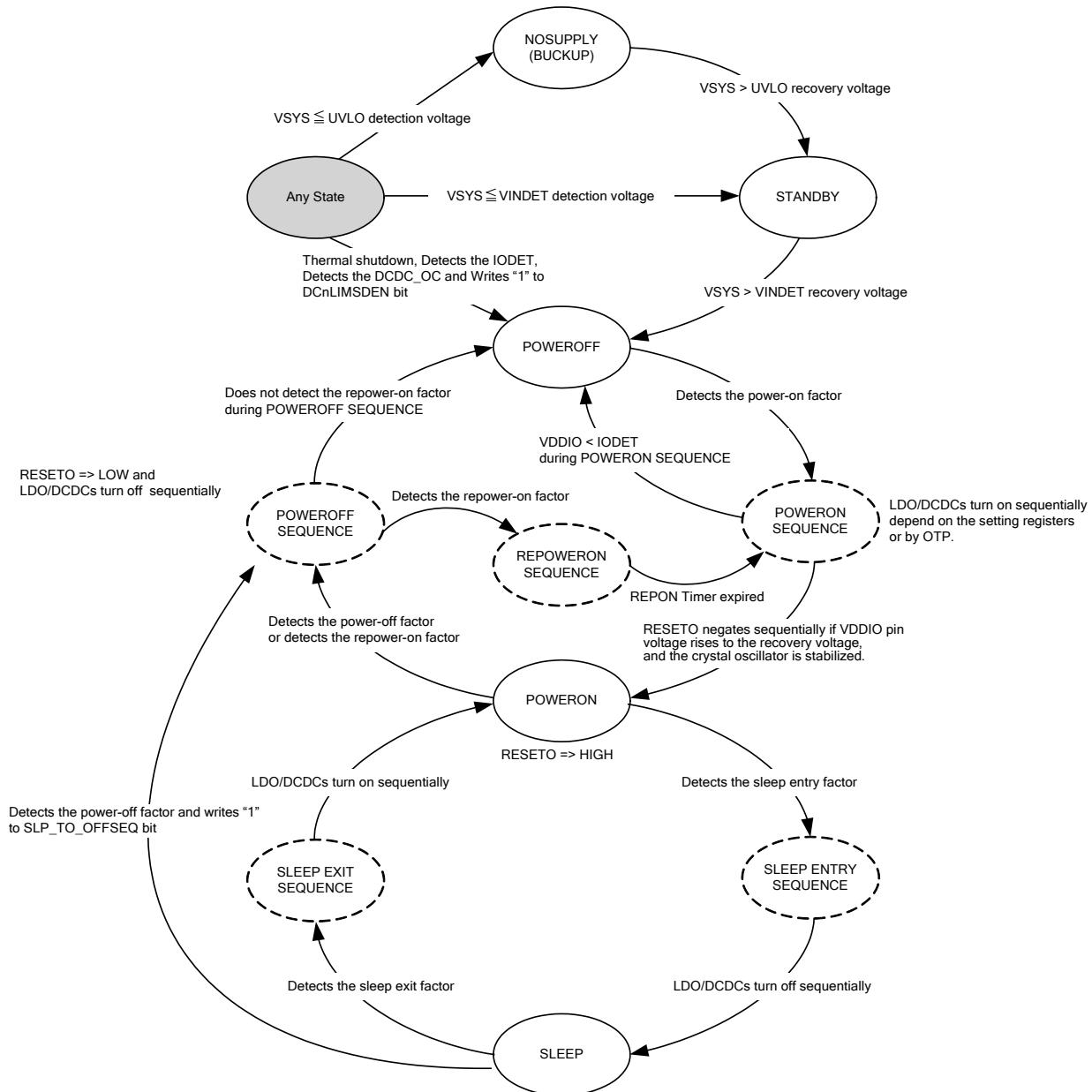
Fig 7-1 Power Control State Machine Diagram
