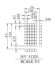
The non-specified tolerance of dimension is  $\pm 0.3 \text{ mm}$ .
