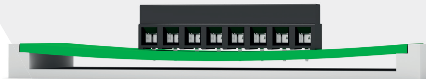
Example of strain between the pins and the PCB
